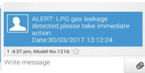
Fig 12: Gas leakage SMS has arrived.
